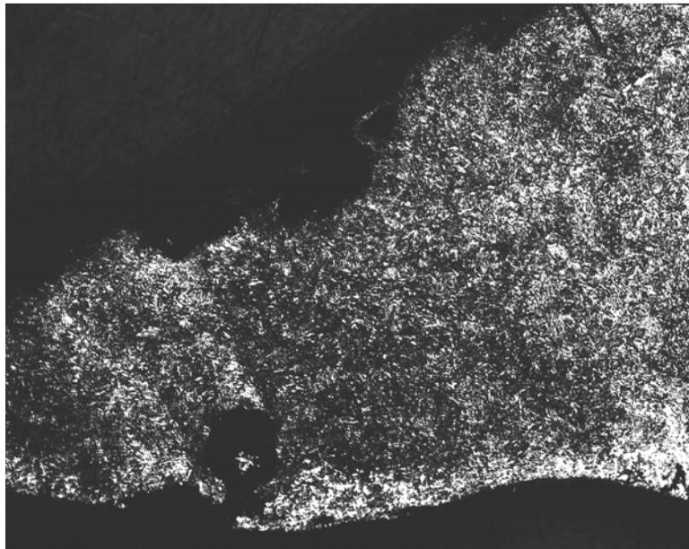
Fig. 9: 1.- Sword A36. 2.- Photomicrograph F1 x 160. Martensite near the edge.
