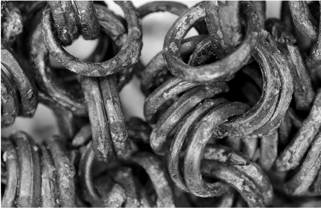
Figure 12. The rings were made by bronze casting in a bivalve mould. The casting seam can still be observed on the outside of the rings (photograph M.A. Wijnhoven).
