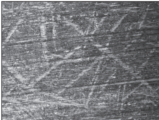
Figure 12. The bottom surface of the 2.7 kg ingot 10x. This ingot is number I. The figure shows when the cooling rate is faster than the furnace cooling. Matrix here shows widmanstätten needles that are Cm (cementite). This happens when cooling rate is too fast Cm to nucleate and diffuse to those carbide-forming elements that are in interdendritic regions. Carbon gets trapped inside the very large grains and forms needle-like structures.
