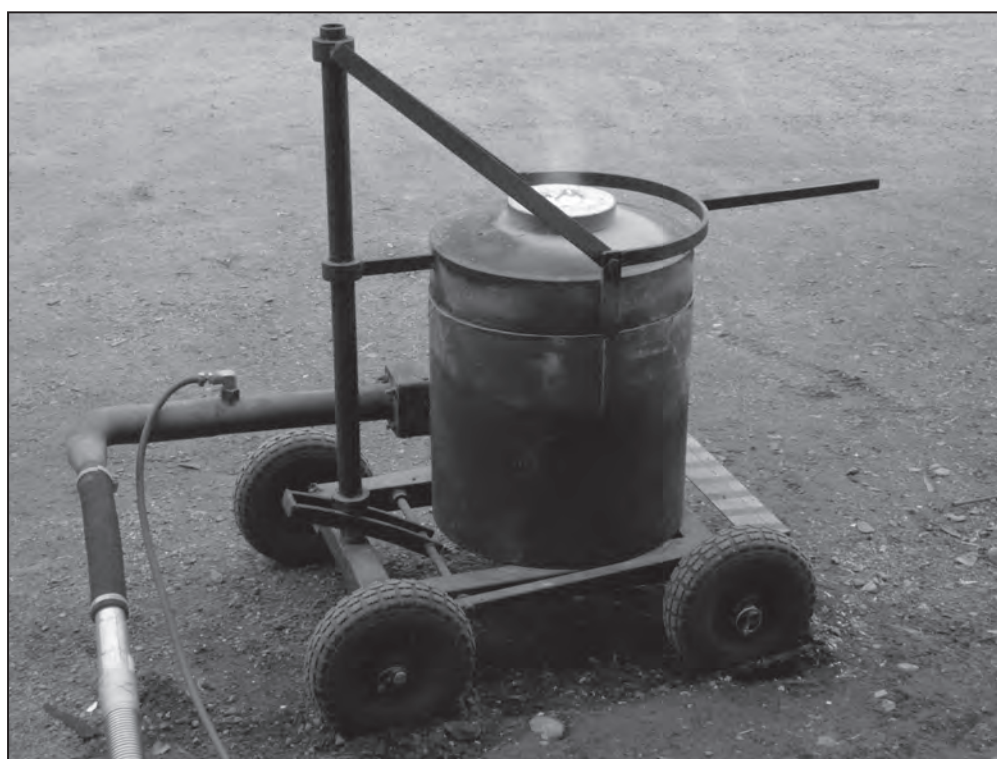
Figures 3-4. A self-made gas/air furnace with a high temperature refractory cement lining and lid.
