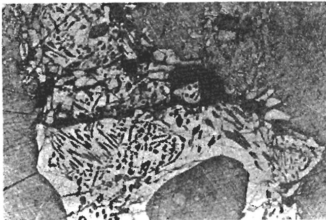
Sample 5  $\times$  800. An area of tin-rich eutectoid ( $\alpha\delta$ ) in a copper-rich matrix. N. B. Two phases are visible in the eutectoid, which is much harder than the matrix, and may have formed at the top of the casting because deliberate late additions of tin caused a higher local tin content. There is also a trace of silver present (detected by electron microanalysis).
