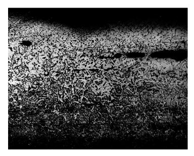
Fig. 13. Cross-section of the upper breastplate. The microstructure consists of ferrite with areas of pearlite along one side.
