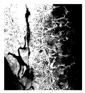
Fig. 11. Cross-section of the left cowter. The microstructure consists of pearlite with a little ferrite.
