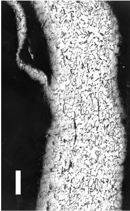
Fig. 10. The microstructure of the visor of Churburg 16; ferrite and pearlite.
