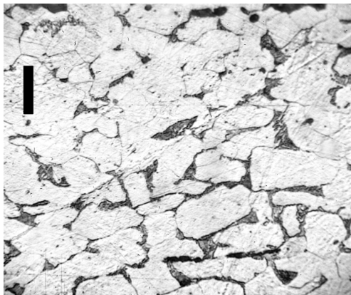
Fig. 11. The microstructure of the visor of Churburg 16 at higher magnification.
