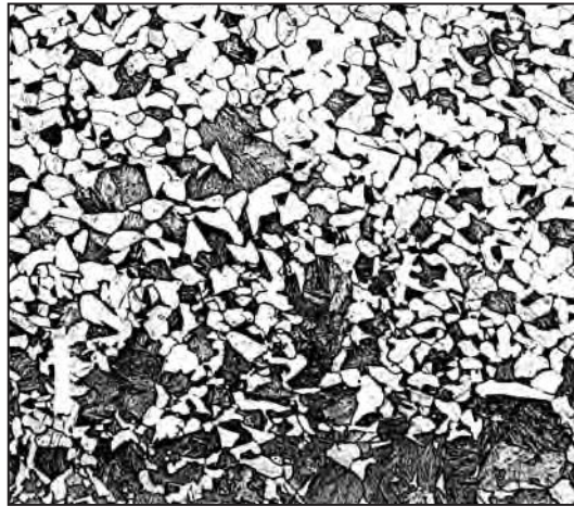
Figure 28. Microstructure of arm (B183); ferrite and low-carbon martensite; scale bar = 75 microns.
