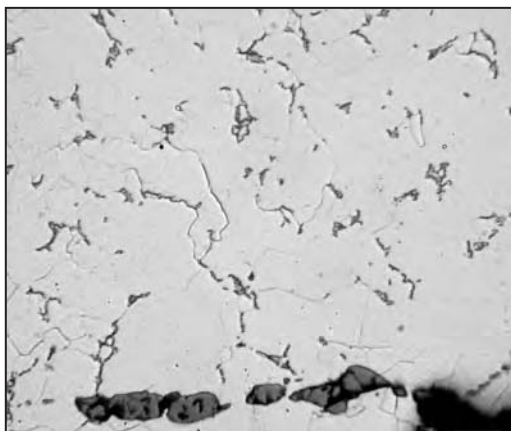
Figure 4. Microstructure of A23 breastplate; scale bar = 50 microns.
