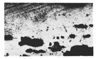
IN. 7006 X 100 64.17 Surface of blade is at top of photograph. Note gradual carburisation.
