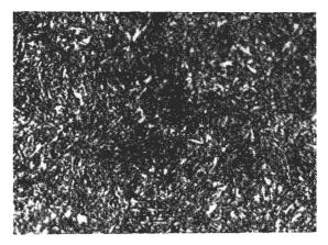
Reheated martensite (?). The carbide particles outline the orignal structure vaguely.
