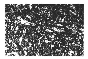
LM. 6369 X 1600 Carbide particles probably formed by heating h 63.21
