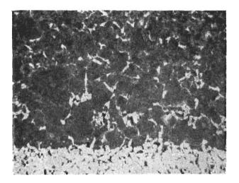
Ea 92 X 192 The border between the high-carbon and low-carbon areas is very sharp.
