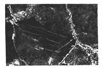
X 1280 71.16 Very fine pearlite and needles of cementite deposited within the pearlite areas. (Area c on section.)
