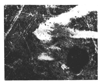
X 320 At the weld. Note slag inclusion, and light streak perhaps left by flux from welding.
