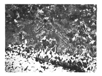
Ea 92 X 240 The bardened zone contains martensite, a dark-etching material, and (near the centre) spiny ferrite. Note the long slag inclusion.
