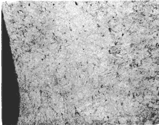
X 100. Note annealing twins and slip lines
