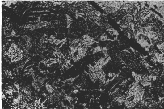
X 500 One of the dark-etching streaks (bainite)
